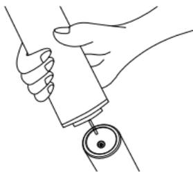
Remove the lid of the refill cartridge / gas cartridge and remove any adaptor ring and adaptors present. Adaptors are not usually necessary for refilling the RÖSLE flambé burner. If by chance the nozzle of the refill cartridge does not fit the gas valve of the burner, select the appropriate adaptor ring.
